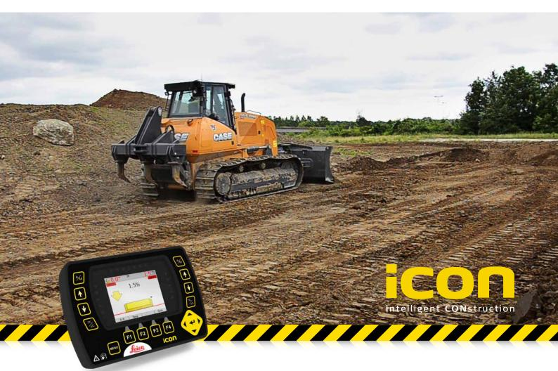
Keeping track of multiple parameters when grading is a thing of the past. With Leica Geosystems' iGD CoPilot, the dozer operator only needs to concentrate on the speed and direction of the machine. The critical factors, cross slope and height of the blade, are adjusted automatically by iGD CoPilot.
